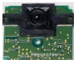
▲ Example in which a photosensor and an optical component are combined (optics module)
