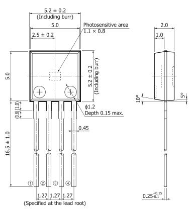
Tolerance unless otherwise noted:  $\pm 0.1$ ,  $\pm 2^{\circ}$ ① GND
