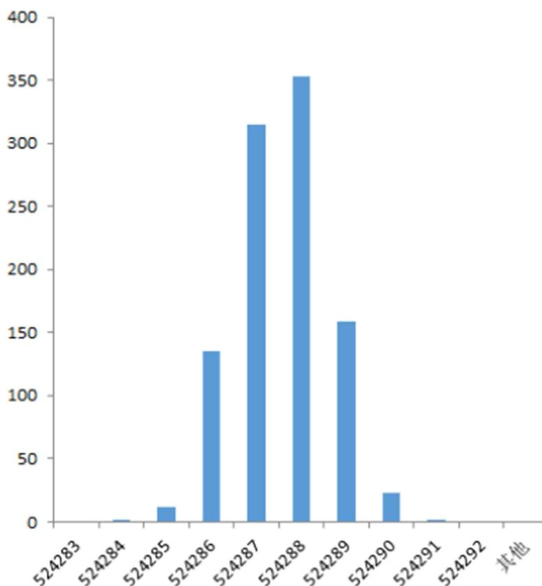
MS5185T 噪声分布柱状图 (AVDD=4V, 内部基准, Gain = 64, Update Rate = 16.7 Hz)
