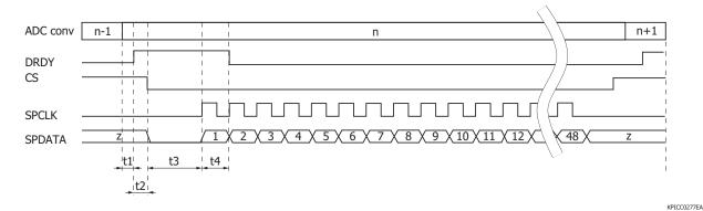
Period Description Min. Max. One internal CLK cycle t1 From the completion of ADC conversion to the rising edge of DRDY  $0.33 \, \mu s$ t2 From the rising edge of DRDY to the falling edge of CS 10 ns From the falling edge of CS to the first rising edge of SPCLK t3 10 ns One SPCLK cycle t4 From the first rising edge of the CPCLK to the falling edge of DRDY 10 ns
