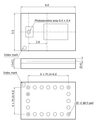
Tolerance unless otherwise noted:  $\pm 0.1$  Chip position accuracy with respect to package dimensions marked \* X, Y $\leq \pm 0.2$ ,  $\theta \leq \pm 0.2$  Values in parentheses indicate reference values.
