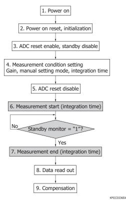
Sensitivity variation can be decreased using the compensation coefficient which is calculated from the integration time measurement result. Explanation of compensation method is shown as follows.
